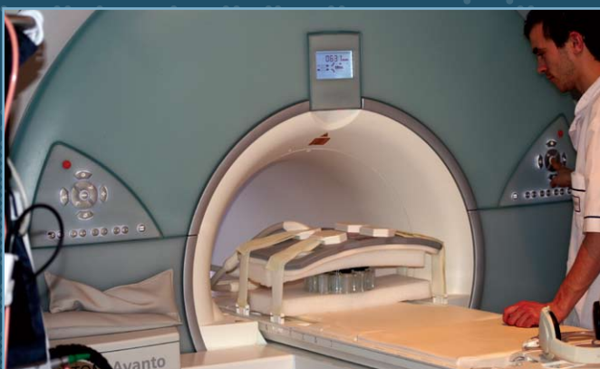
Eurospin Test Object n°5 consists of test tubes made of agarose doped with Gadolinium corresponding to different concentrations and therefore T1 values (Middle), placed in a magnet (Bottom)
